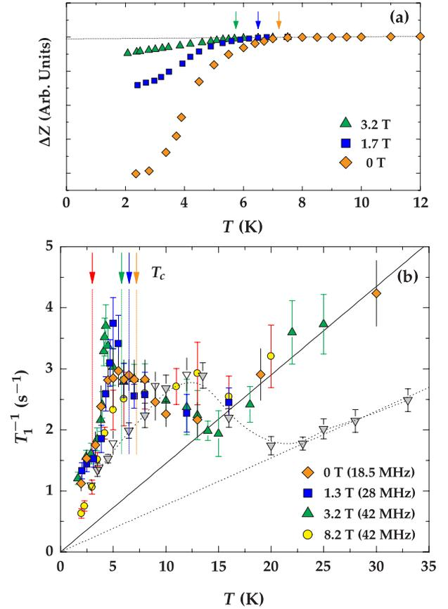
FIG. 3 (color online). (a) Loss of impedance  $\Delta Z$  due to superconductivity measured in NMR tank circuit at 0.5 GPa. Down arrows denote  $T_c$  for each field. (b)  $^{75}\text{As}$   $T_1^{-1}$  versus  $T$  at  $P = 0.5$  GPa. Down triangles are data taken at ambient pressure at 45 MHz (closed: 3.6 T, open: 8.8 T).
