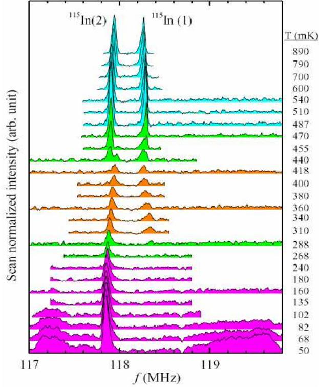
**Fig. 1.7.** NMR spectra of In(1) and In(2) transitions in CeCoIn<sub>5</sub> at 11.1 T. In (1) transition shifts down in frequency, whereas the In(2) shifts up in frequency.
