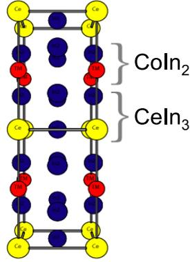
**Fig. 1.1.** Crystal structure of CeCoIn<sub>5</sub>, showing the layers of CeIn<sub>3</sub> and CoIn<sub>2</sub>.
