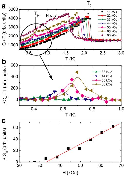
Fig. 2. (a)  $C/T$  versus  $T$  at 1.95 GPa for  $H \perp ab$ -plane. (b)  $\Delta C_M/T$  after subtracting smooth varying superconducting background. (c) Entropy involved in the field-induced magnetism plotted as a function of field  $H$ . Solid line is a guide to eyes.
