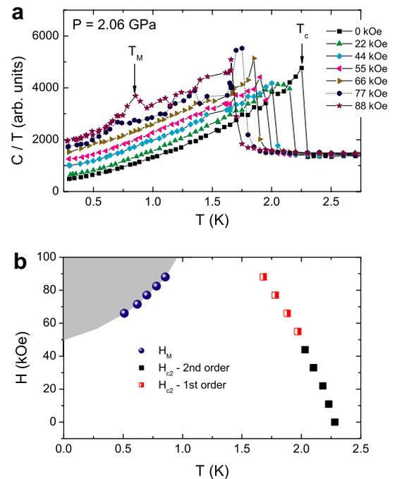
Fig. 3. (a)  $C/T$  versus  $T$  at 2.06 GPa for  $H \perp ab$ -plane. (b)  $H$ - $T$  phase diagram based on specific heat measurements.  $H_M$  represents the critical field to induce magnetism in the mixed state. Filled (half-filled) squares display second-order (first-order) upper critical field  $H_{c2}$ .
