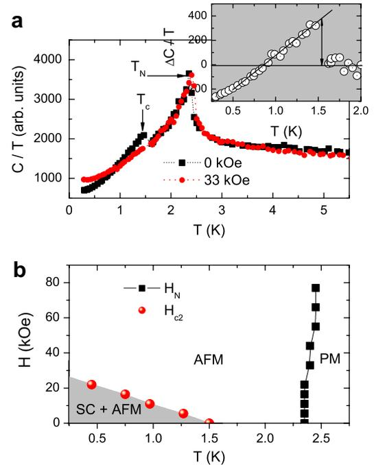
Fig. 1. (a)  $C/T$  versus  $T$  for  $H=0$  (squares) and 33 kOe (circles) at 1.6 GPa.  $T_c$  and  $T_N$  represent superconducting and antiferromagnetic transition temperatures, respectively. Inset:  $\Delta C/T$  versus  $T$ , where  $\Delta C = C(0\text{ kOe}) - C(33\text{ kOe})$ . Solid lines are guides to eyes. (b)  $H$ - $T$  phase diagram at 1.6 GPa. PM and AFM indicates paramagnetic and antiferromagnetic state.
