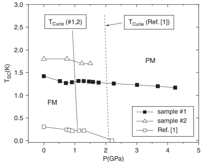
Fig. 3. Pressure dependence of superconducting transition temperature of  $\text{ZrZn}_2$ .
