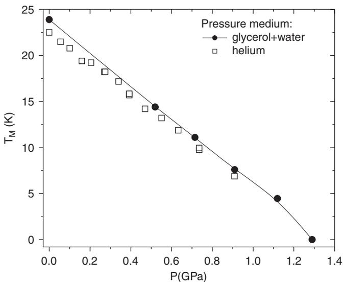
Fig. 2. Pressure dependence of the Curie point of  $\text{ZrZn}_2$ .
