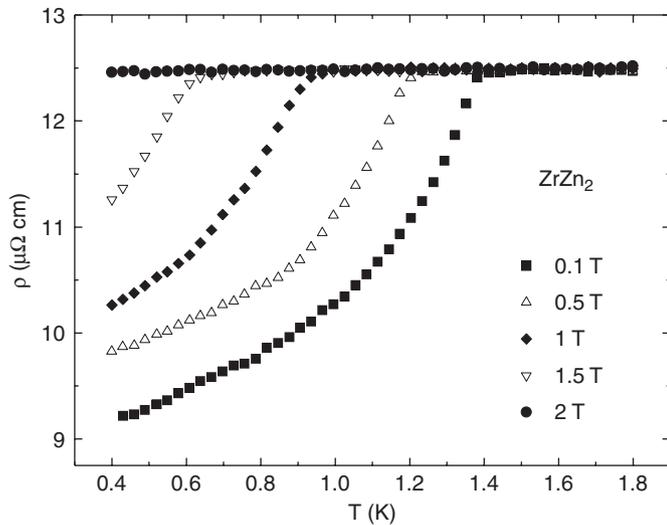
Fig. 1. Low-temperature resistivity of  $\text{ZrZn}_2$  sample, having a Curie point  $T_C = 25$  K, as determined by AC susceptibility and Arrott plots in magnetization measurements.
