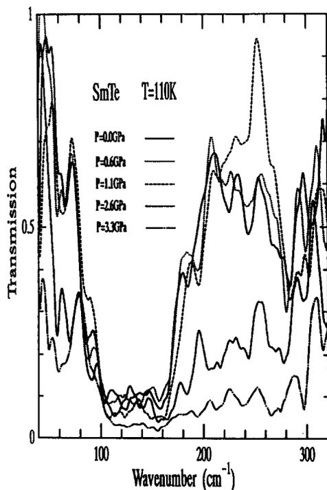
Fig. 3. The wave number dependence of transmissions under several pressures at 110 K for SmTe.
