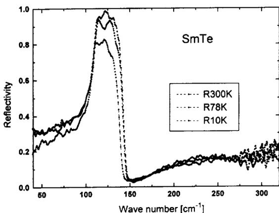
Fig. 1. The wave number dependence of reflectivities at 300, 78 and 10 K at  $P = 0$  GPa for SmTe.
