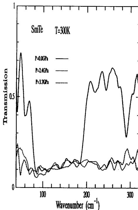
Fig. 2. The wave number dependence of transmissions under several pressures at 300 K for SmTe.
