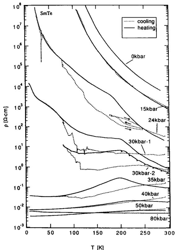
Fig. 4. The temperature dependence of electrical resistivities under several pressures for SmTe.
